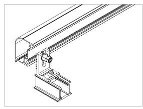
**ATTACH TRIMRAIL TO ROOF ATTACHMENT:** Attach rail using 3/8" hex bolt & Tri-drive or serrated flange nuts. Make sure Trimrail<sup>™</sup> is level across all Trimrail<sup>™</sup> roof attachments. After rail is level, tighten channel clamp bolts to secure Trimrail<sup>™</sup> roof attachments to channels.
