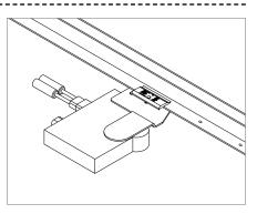
LIFT MODULE AND DISCONNECT MLPE CABLES
