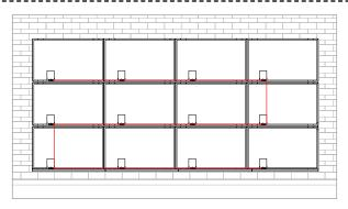
**MICROINVERTER:** Before installing a row of modules place microinverter trunk cable.
