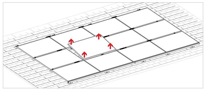
Bonding note: If both sides of array are bonded with NS Bonding Clips, as recommended, then no additional bonding is required for module maintenance.
